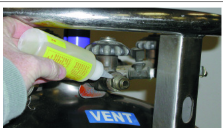
Oxygen Safe Valve Leak Check
