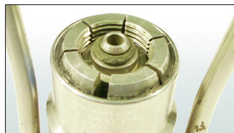
Figure 18. An example of a "bad O-ring" main seal.
