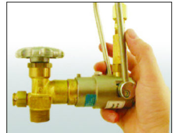
Figure 4c - 4d. Align the CGA 580 tight and square against valve with no visible gap. Align the CGA 580 RPV with valve to avoid damage to the sealing surface.
