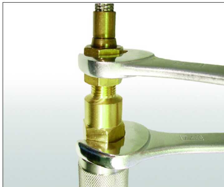
Figure 1. Torque to maximum 15 ft-lb.
