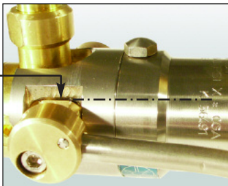
Figure 11. Cams are square to sleeve.
