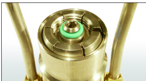
Figure 17. An example of a "good O-ring" main seal.
