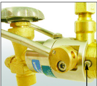
Figure 13. Safety pin extends to stop sleeve travel and accidental disconnection.
