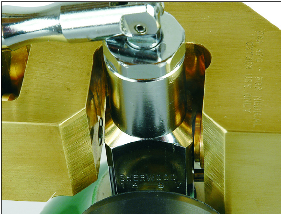
Figure 8. Valve properly aligned.
