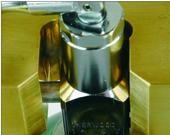
Figure 12. Valve is tight to the body.
