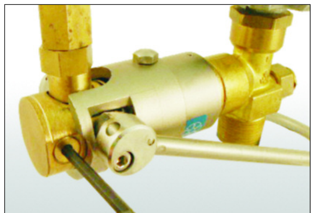
Figure 28. The retaining screw has to be tightened to a torque of 2.5 ft-lb using a 4mm hex key and a calibrated torque wrench. Ensure that all parts are cleaned before reassembling the connector. (See torque wrench, Figure 19).
